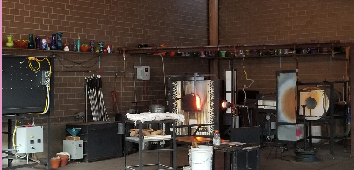
A glimpse into the “hot shop,” or glass blowing studio, of Galen Tisselly. A furnace, “glory hole” for reheating works-in-progress, and many metal rods, wooden paddles, and other instruments for inflating and shaping blown glass.
